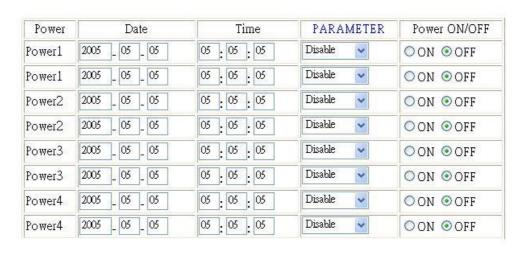
If user wishes to control the power in one outlet of IP Power 9258, you can fill in the time in the power control column and choose on or off.
